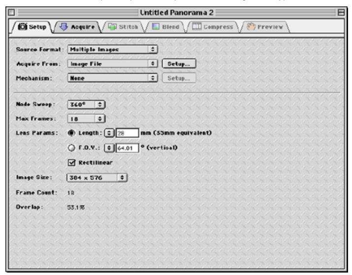
The "Setup" panel is where information about your camera and source images are supplied. In this case, we've taken 18 photographs using a 28mm lens for a 360° panorama. The photos were scanned on a flatbed scanner yielding a 384 x 576 pixel image.
